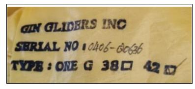
Figure 7: Rescue parachute nameplate
