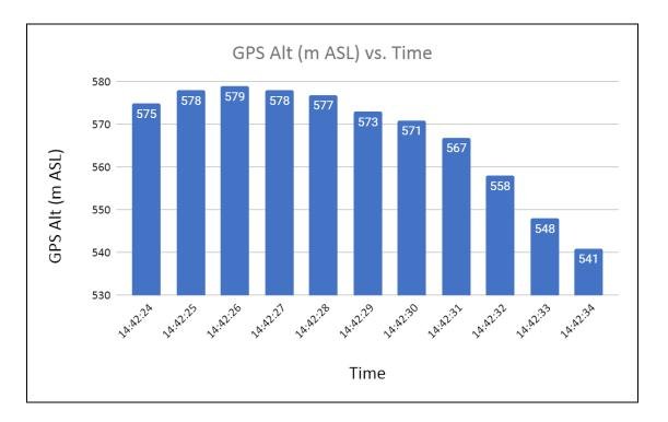
Figure 20: Tracklog derives GPS altitude for the last 10 seconds of flight. Rapid loss of altitude starts from 567m ASL. The accident occurred at 541m ASL.
