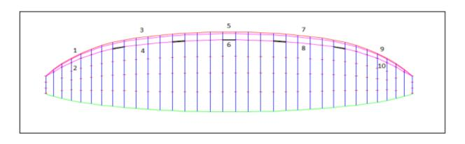
Figure 25: Porosity test locations
