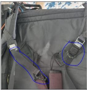
Figure 22: Harness setup showing leg straps asymmetry
